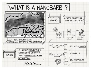
BNNano uses a proprietary, catalyst-free process, to manufacture an enhanced boron nitride nanotube called the Boron Nitride NanoBarb<sup>™</sup>, with properties enhanced beyond typical nanotubes further making the NanoBarb<sup>™</sup> a strategic component for improving advanced materials.
